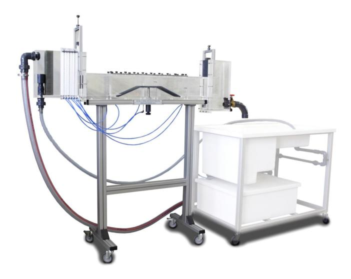
To study the behavior of fluids in open channels and closed conduits, performing a wide range of experiments with open channel or closed conduit.
